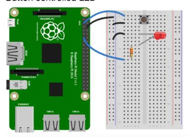
Turn on an <u>LED</u> when a <u>Button</u> is pressed:
